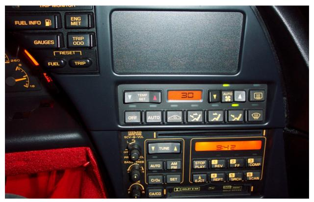
• The displayed value x25 = the idle speed. 30 x 25 = 750. In this case the idle speed is 750 rpm.
