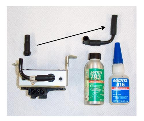
The connector can be reattached or replaced with 3/16" vacuum hose.
