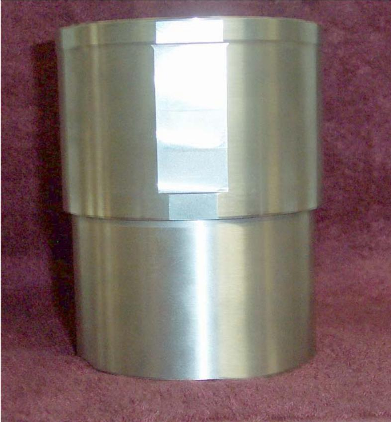
The top half of the liner is thicker than the bottom half so thermal and mechanical loads on the liner cause it to expand and contract different amounts between the top and the bottom. The liners are from Mahle in Germany. The liners were dropped into the block during the assembly. The cylinder heads clamp the liners into the block. It is not possible to hone a Nicasil bore so the liners can't be finished for best straightness after they are clamped in the block.
