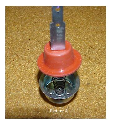
Picture 4 shows the normal position of the return spring.
