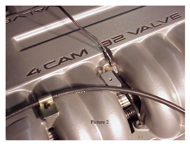
runners. In picture 2, the lamp of a light tool is ready to be lowered into the left side valley area.
