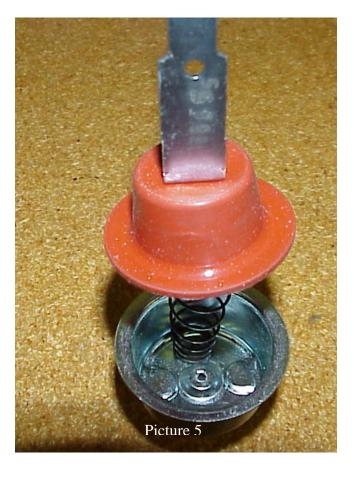
Picture 5 shows the position of the spring, if the unit is improperly assembled.
