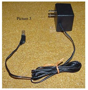
Picture 3 shows the light tool. The tool can be constructed from a 12 volt power supply and a #168 automotive accessory light bulb. A flashlight will do, but it is not as cool or as effective as the small lamp on the wire. The secondary actuator verification procedure:
