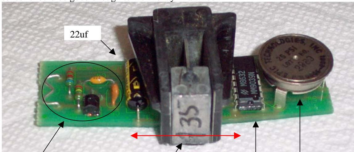
RF Transmitter. The piezo armature vibrates in the gap.
