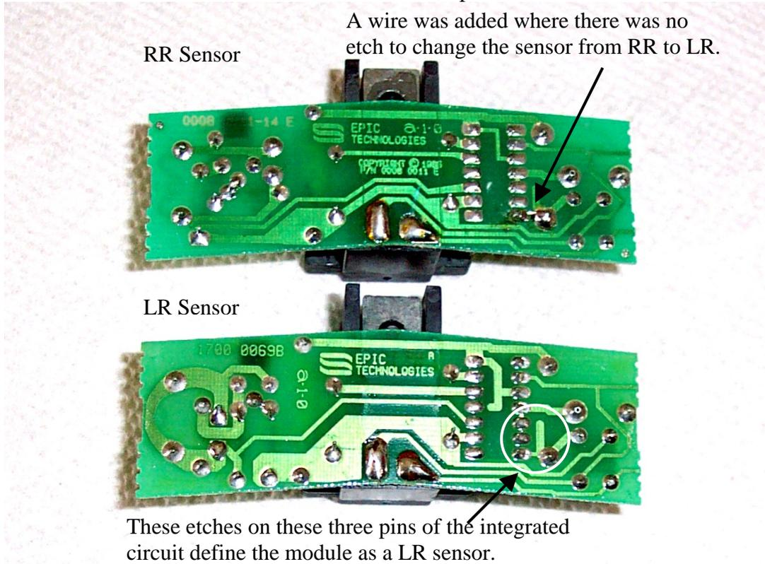
The receiver module on a '92 car can be used to verify that the modification was performed correctly. The '92 receiver can identify which module is signaling a low tire pressure condition. The codes are 23 for the RR, 33 for the LR, 43 for the LF and 53 for the RF. The '91 service manual lists these low tire pressure codes for the '91 cars. However they don't function on a '91.
