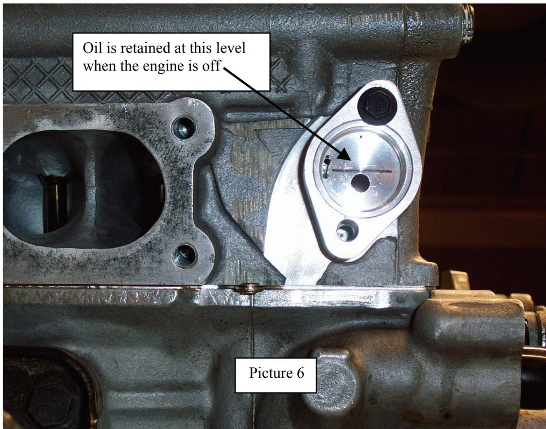
In picture 6 a line has been drawn to show the upper level of the oil that is retained in the tensioner housing when the engine is off. Because the oil galley inlet has been raised, oil remains in the tensioner holder when the engine is off. This way the oil inlet check valve for the tensioner is always covered with oil. When the engine is cranked, oil is available immediately for the tensioner to draw-in until the oil galley refills with oil.
