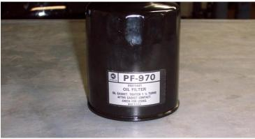
The Bosch Premium 3401 oil filter is a good choice for the LT5. The anti-drainback valve works very well and it has filtration and flow characteristics that are compatible with the PF970C. The manufactures provided the following performance specifications for the original PF970C (early filter) and the Bosch 3401. The testing was performed according to SAE specification HS-806.
