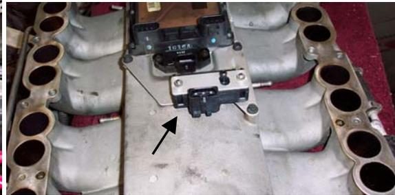
The secondary vacuum pump cycle time can be used as a diagnostic to locate leaks. If the pump can cycle off for one second the vacuum connections are tight enough for the secondary port throttles to operate correctly. There are four common leakage points in the vacuum lines before the secondary solenoid vacuum valve.
