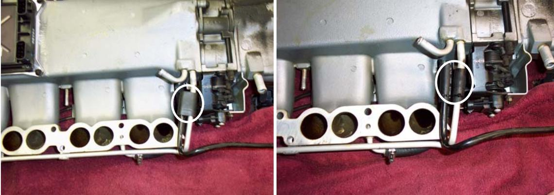
Bend the front tube forward a little to create some space between the tubes. Lubricate the ID and OD of the hose and slip it on the plenum. It fits very tight and does not need a clamp. Slip the two vacuum lines in the hoses and clamp them with plastic ties.
