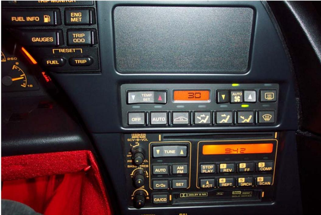
The 30 in the display represents 750 rpm.  $30 \times 25 = 750$  rpm.
