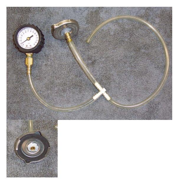
Pinch off the upper 3/8" ID hose on the surge tank. This is the overflow hose that goes to the white reservoir tank. Attach the pressurization tool to the surge tank and use shop air to pressurize the system to 15 psi. After a two second blast of air you will find the surge tank empty, a gratifying sign of progress. The system will fill normally to the top after that. Start the engine and observe the glory of the coolant flow out of the surge tank air bleed tube.
