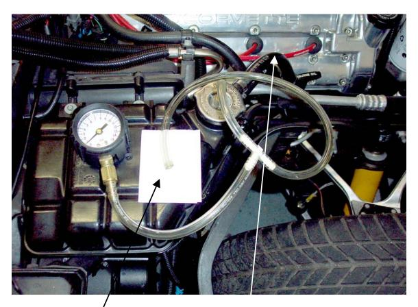
Apply shop air here. Pinch off the overflow hose here.
