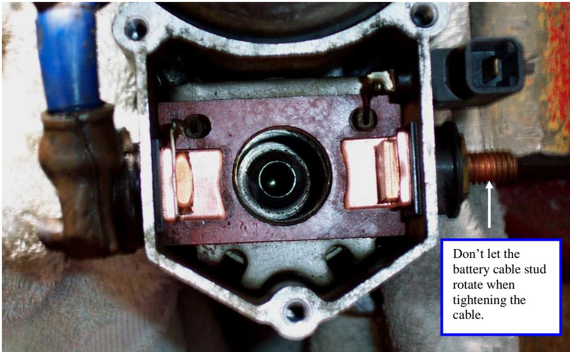
The contacts need to be level and square with the housing so that the plunger contact disk will lie evenly across them and make contact across the full faces of the contacts. The battery terminal stud does not have an anti-rotation stop. If it moves when tightening the cable, it will lift the corner of the contact. Then the plunger will make a point contact rather than a full-face contact. This leads to shortened contact life and potentially a click and no cranking failure.
