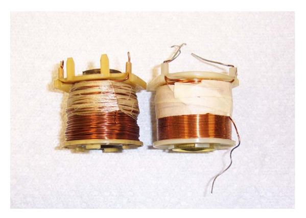
The coil on the right is a new replacement part coil. It is smoothly wound. Maybe the smoothly wound coil is more durable.
