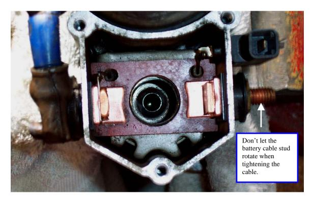
The contacts need to be level and square with the housing so that the plunger contact disk will lie evenly across them and make contact across the full faces of the contacts. The battery terminal stud does not have an anti-rotation stop. If it moves when tightening the cable it will lift the corner of the contact. Then the plunger will make a point contact rather than a full-face contact. This leads to shortened contact life and potentially a click and no cranking failure.
