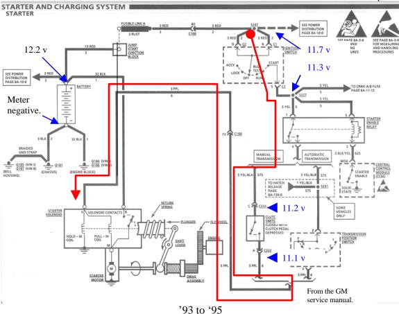
In '93 GM improved the starter solenoid circuit wiring. The clutch switch connections were moved to the armature side of the start relay. This reduces the load on the clutch switch from 30 amps to .2 amp. It also eliminates the approximately .050 volt normal voltage drop across the clutch switch and its wiring at 30 amps.
