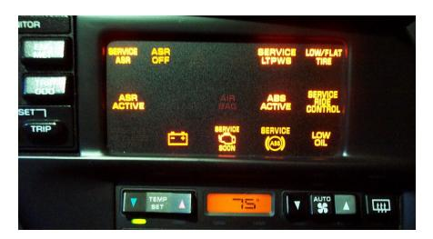
This display is for a '94 car. '92 to '95s are the same except for detail differences in the Service Engine and Service ABS icons.
