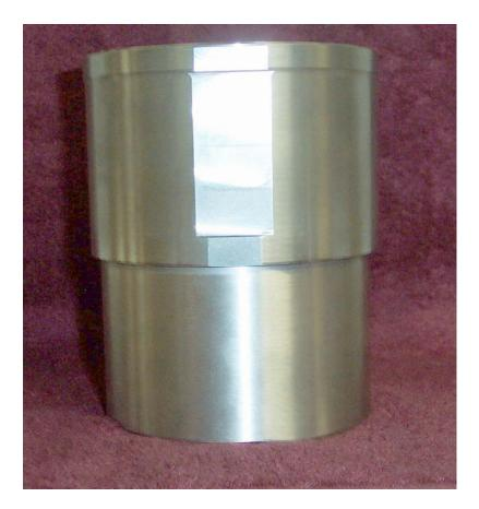
The top half of the liner is thicker than the bottom half so thermal and mechanical loads on the liner cause it to expand and contract different amounts between the top and the bottom. The liners are from Mahle in Germany. The liners were dropped into the block during the assembly. The cylinder heads clamp the liners into the block. It is not possible to hone a Nicasil bore so the liners can't be finished for best straightness after they are clamped in the block.
