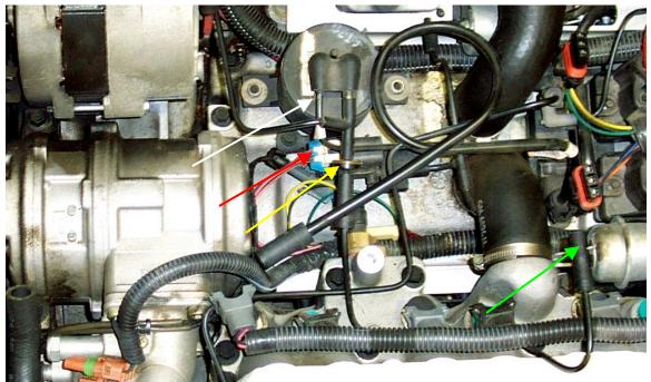
After determining that the vacuum connections are tight before the vacuum solenoid valve, test the connections after the valve. The valve can be opened by grounding pin C17 at the ECM. The "C" connector is the green ECM connector. The pin locations are marked on the connector in very small print. The wire is pink with a black stripe on all model years except for early '90's where it is red.
