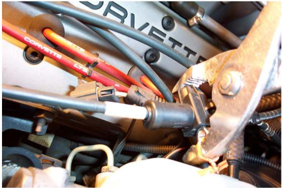
Depressing the cable length adjuster. The button is the flat section.
