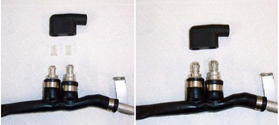
To sleeve the valves, slip short stubs of <sup>1</sup>/<sub>4</sub>" vinyl tubing on the nipples. Secure the grommet to the PCV tube with a <sup>1</sup>/<sub>4</sub>" wide worm gear clamp just as GM did beginning in '93. Install a plastic tie to hold the grommet down. Clamp it lightly so that the hose that the PCV valves are mounted on does not get crimped at the bottom.
