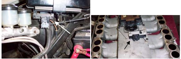
The secondary vacuum pump cycle time can be used as a diagnostic to locate leaks. If the pump can cycle off for one second the vacuum connections are tight enough for the secondary port throttles to operate correctly. There are four common leakage points in the vacuum lines before the secondary solenoid vacuum valve.
