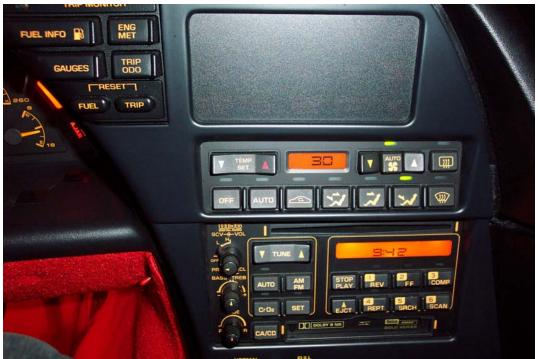
The 30 in the display represents 750 rpm.  $30 \ge 25 = 750$  rpm.
