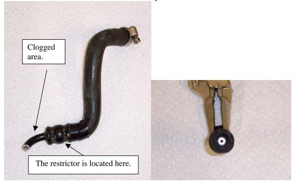
The radiator air bleed flow restrictor. Left, the hose after being cut from the tube. Right, the restrictor after cutting the hose. This hose would not flow with 90 psi of air pressure applied.
