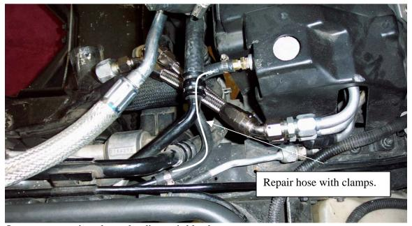
One way to repair a clogged radiator air bleed.
