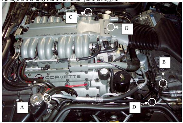
Diagram of the air bleed system. This engine has a throttle body coolant bypass line. Normally the hoses connect to the right and left of the plenum where the tubes are capped in the picture.
